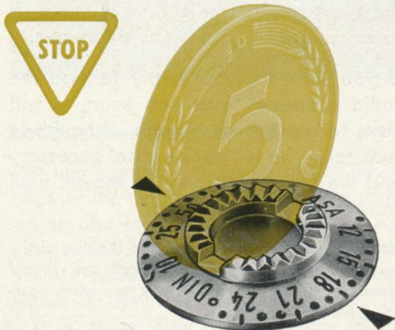
Before taking any photographs remember to set the speed of the film on the camera to be sure of correctly exposed photographs. The film speed disc is turned by means of a coin until the required
